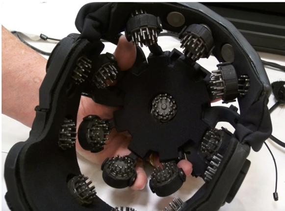
This piece of high-tech headgear was originally designed for the military, but is now in the commercial research market. It is wireless, allowing the subject to move freely. For example, the GIVER wore the DSI-24 while they administered the Bars session. The electrodes on this unique headgear are shielded, much like a “Faraday Cage” that filters out unwanted frequencies in the atmosphere that can interfere with good quality EEG data capture.
